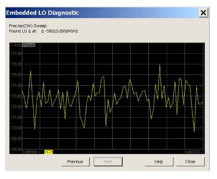
Figure 11. After updating the reference LO, the phase change shows that the estimated DUT LO frequency is still off by about 1 Hz (default tolerance). Perform VMC at this reference LO frequency.
