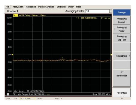
Figure 6. Orange trace = DUT embedded LO locked to reference mixer LO source. Yellow trace = Using Embedded LO Measurement Option (option 084).
